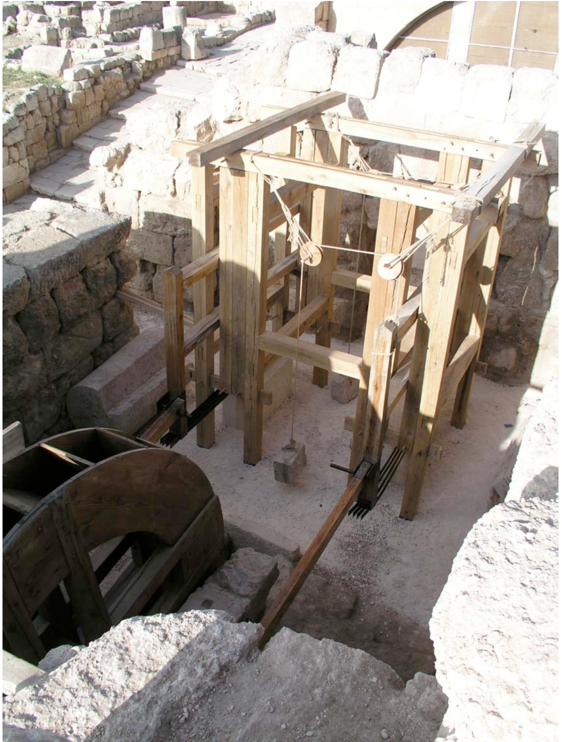
Jerash water saw reconstructed by the Ecole Lycée Professionel Emile Delataille at Loches near Tours, France. Photo courtesy of Dr. Jacques Seigne.
